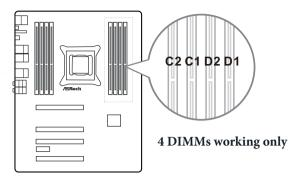
When installing memory modules, the DIMM slots should be populated in the following order: DDR4\_C1, DDR4\_D1 and then DDR4\_C2, DDR4\_D2.
